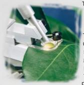
The PAR / temperature leafclip facilitates measurements made under ambient light conditions.
