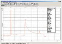
PC-control from Modfluor32 Windows<sup>®</sup> software allows real-time trace plotting as a chart-recorder emulation with calculated parameters written to a text parameters window. Instrument features and parameter measurement routines are selected from
